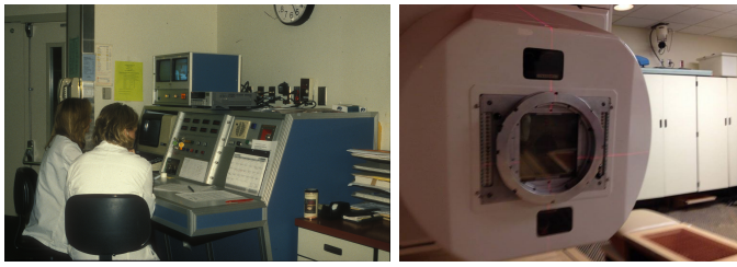
■ Figure 1 The CNTS console, collimator, and patient setup in gantry.
