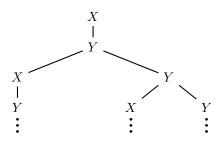
The branches of this unique tree are exactly the executions of the transition system. As a consequence, any LTL formula holds on all executions of the transition system if and only if it holds (with probability 1) on all branches of the generated tree.
